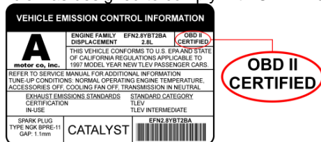
Fig. 1 - Vehicle Emission Control Information Label
